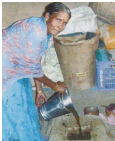
Sindhutai Tayade adds cow dung slurry to her plant through the feeder
