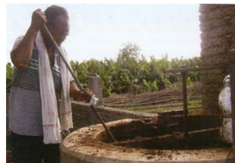
Vijay Ingle stirs the slurry in the biogas digester plant
